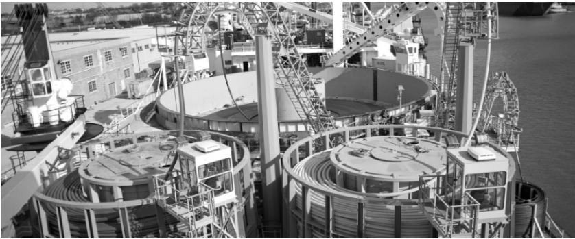
Cable Carousels aboard Cable Laying Vessel Julio Verne
